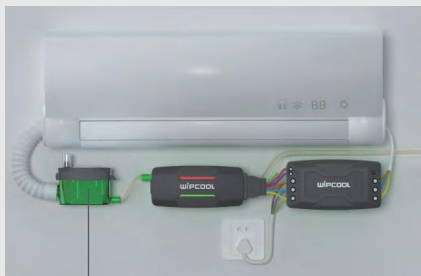
Failure drainage status-Output was cut off when water reaches alarm level to trigger safety switch. To prevent refrigeration equipment from continuing to generate condensate water
